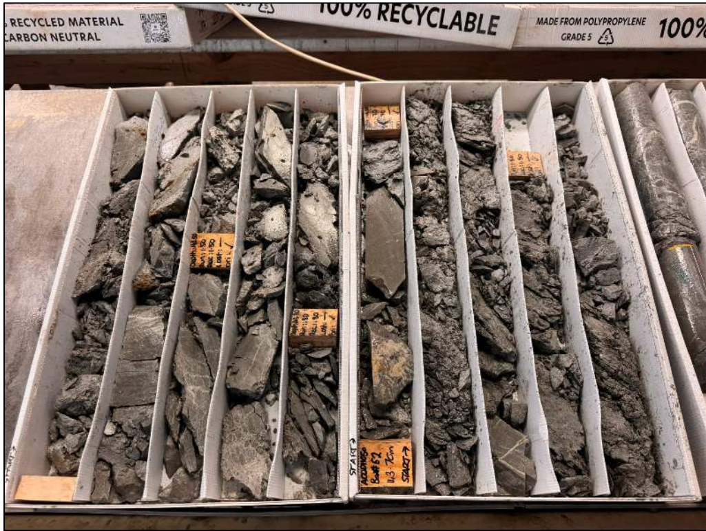
Figure 12-1: Example of core tray verification conducted by the QP (ACDDH050: Box 61 and Box 62).
