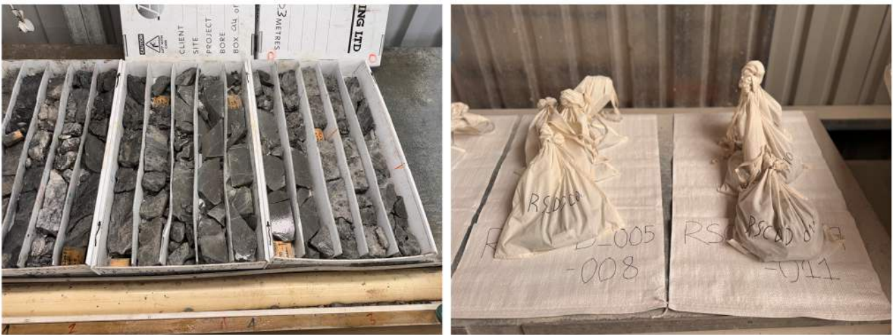
Figure 12-8: Half-core verification samples prior to cutting (left); quarter-core check samples relabelled (right).
